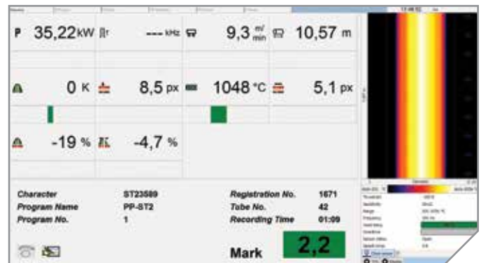
GUI during welding with automated seam evaluation.
