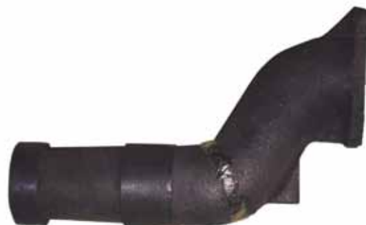
Exhaust outlet. No spares available. Repair necessary.
